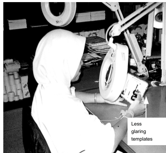
Figure 3b. Ergonomic improvement: the glare from the inspection templates was reduced by changing to a less reflective material.
